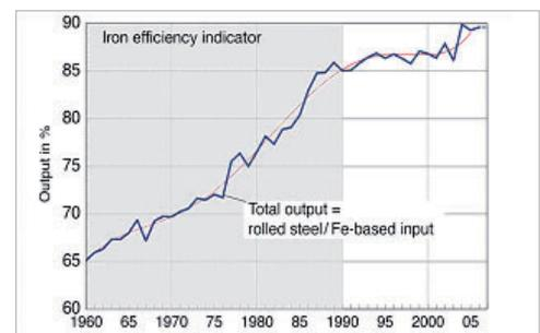
Figure 2: Iron efficiency indicator of the German steel industry
